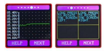
This interface is voltage measurement waveform diagram. It automatically changes the range within the range of 4.5-24V measurement and displays voltage fluctuations in real time.
