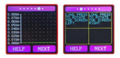
This interface is the current measurement waveform diagram. It automatically changes the range within 0.00A-3.00A measurement range and displays current fluctuations in real time.
