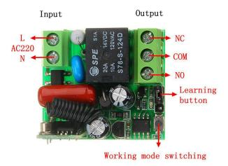
Basic connection of learning type 220 volt single remote control switch AK-RK01s-220 1, connected to 220 volt AC output diagram, as shown below
