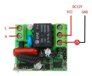
As shown in the figure above, the learning type 220V single remote control switch AK-RK01S-220 input terminal, connected to a 220 volt AC power supply. The common end of the output terminal is connected to the positive pole of the DC power supply, and the positive pole of the appliance is connected to the normally open end, and the negative pole is connected to the
