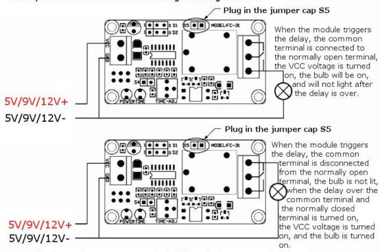
Plug in S5, the common terminal of the relay is connected with VCC, and the relay can directly control the on and off of VCC voltage.
