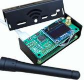
Specifications 802.11 b/g/n wireless LAN 1GHz, single-core CPU 512MB RAM Micro USB power installed JumboSPOT UHF(430-440)+VHF(144-146) (VHF is not the main band, performance reduction)RF extend board. 8G TF CARD Installed PI-STAR panel support DMR,YSF,P25 mode to QSO with RF To internet OLED Display
